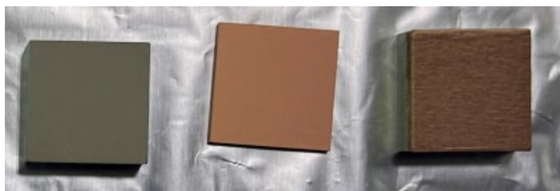
Figure 1. Photo of specimens used in current study. Specimens from left to right are: SS304, Cu, LC-Cu.
